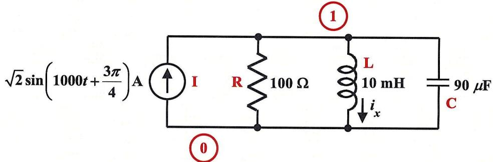
the following LTspice netlist can be used determine the magnitude and phase angle of the steady-state AC part of  $i_x$ :
